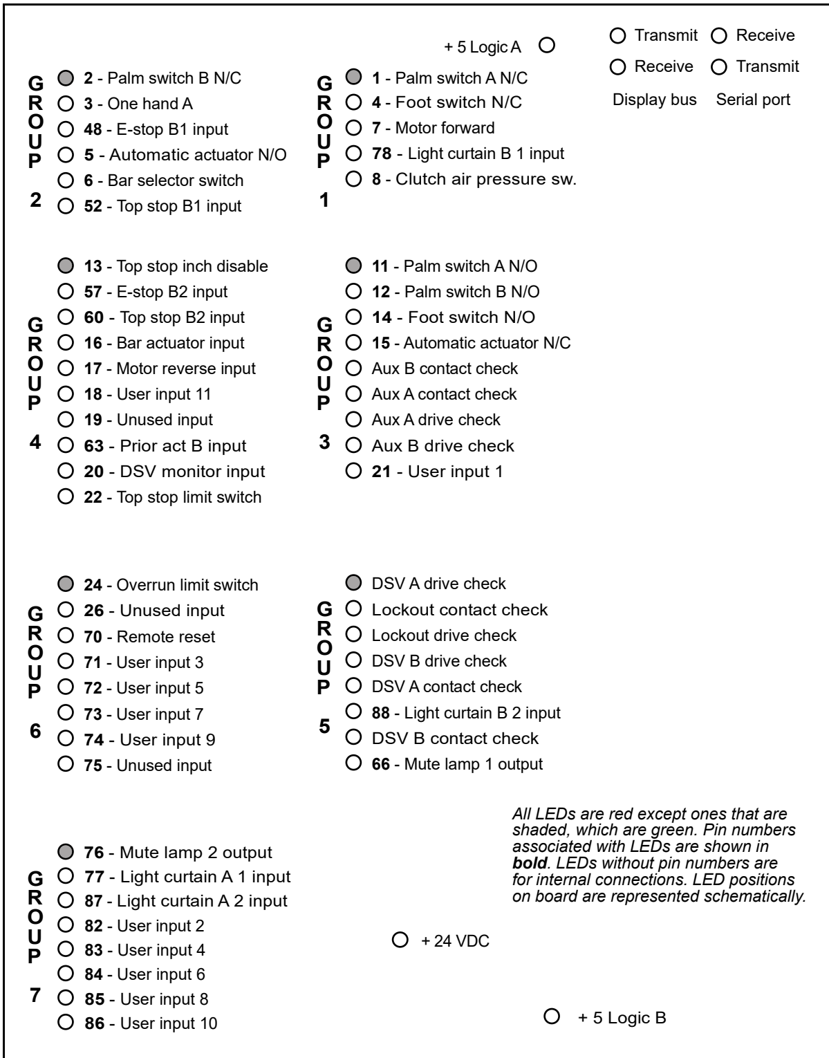
Figure 2-13. LED Map, WPC 2000 Main Processor Board
