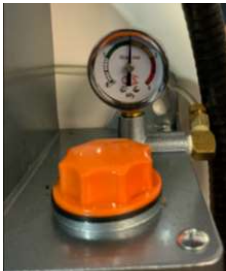
Figure 9 - Properly adjusted oiling system
