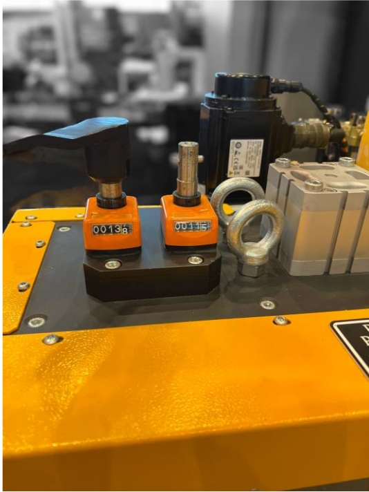
Straightener adjustment made with handles. Mechanical readout for straightener
